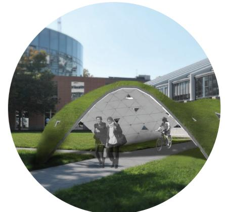
Rendering of proposed on-campus walkway utilizing digitally designed ceramic components
